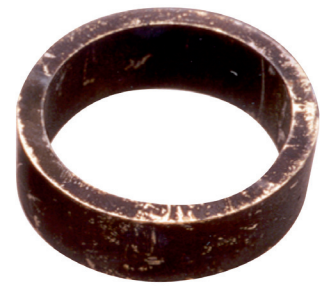
Destroyed by chemical attack due to the incompatibility of different additive systems in the mixed hydraulic fluids
